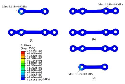
Fig. 4 Pressure on miniplate as the result of loading by (a) MF-42, (b) MF-44, and (c) MF-24 configuration
