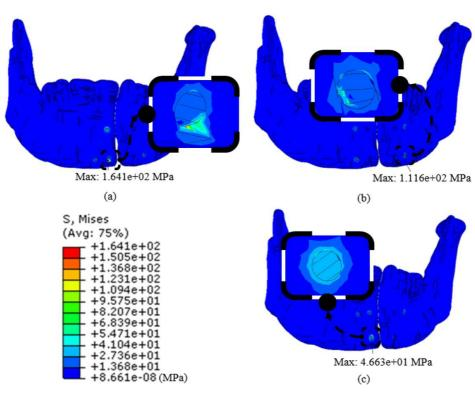
Fig. 3 Pressure occur in screw hole on bone surface by (a) MF-42, (b) MF-44, and (c) MF-24 configuration
