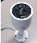
Fig. 3 IR CCTV camera and DVR system
