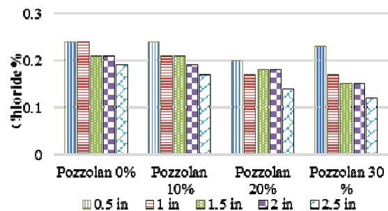
Fig. 14. Chloride Content after 56 Days Ponding Period
