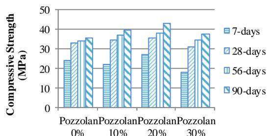
Fig 4. Comparison of Compressive Strength Test Results of Pozzolan 0% to 30%.
