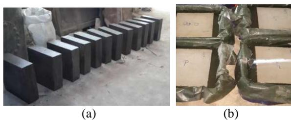
Fig 3. Preparation of Samples for Chloride Penetration Testing, (a) Slabs are Coated with Epoxy; (b) Slabs are Ponding with 3% NaCl Solution
