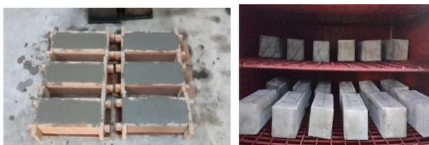
Fig 2. Preparation of Samples for Carbonation Testing
