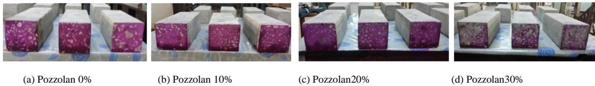
Fig. 5. Carbonation Area Measurement of Samples in Chamber at Age 28 Days
