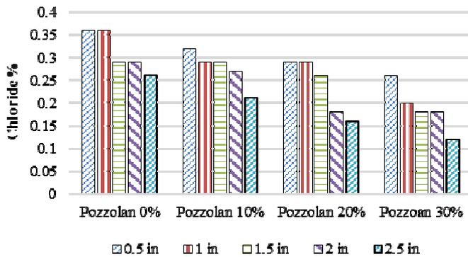
Fig. 15. Chloride Content after 90 Days Ponding Period
