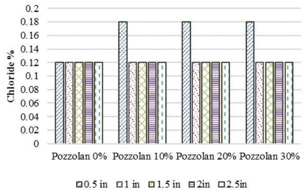
Fig. 13. Chloride Content after 28 Days Ponding Period
