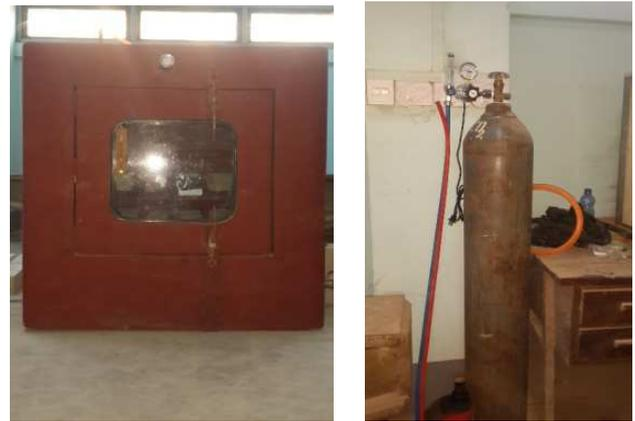
Fig 1. Carbonation Test Chamber
