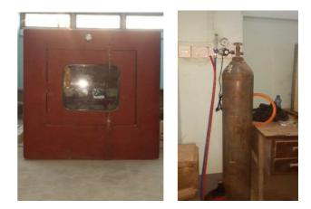
Fig 1. Carbonation Test Chamber
