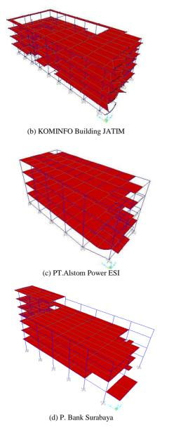
Fig. 7. Numerical Modelling Using SAP 2000 for 4 case studies
