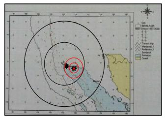
Fig. 12 Seismicity and source zone (epicenter) within a radius of 300km from Andaman earthquake (M=9.1, 2004) and radius 4km from Pidie Jaya earthquake (M=6.4, 2016).
