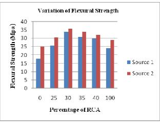
Fig. 4 Comparison of 28 days Flexural strength
