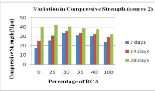
Fig. 2 Compressive Strength test results from source 2
