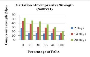
Fig. 1 Compressive Strength Test Results from Source 1
