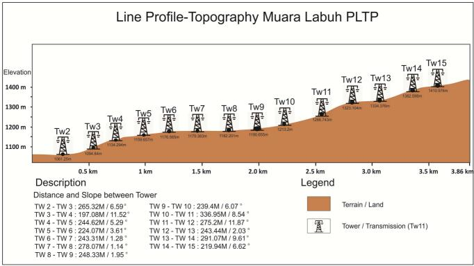
Fig. 6 The profile of topography survey location for the transmission tower recommendation point location
