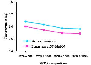
Fig. 5 The effect of SCBA content on concrete mass with w/c = 0.275 (MgSO<sub>4</sub> = 5%)
