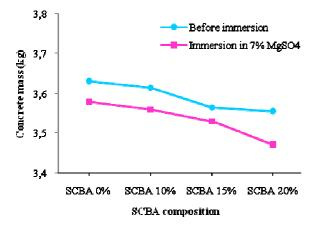
Fig. 10 The effect of SCBA content on concrete mass with w/c = 0,325  $(MgSO_4=7\%)$
