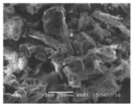
Fig. 1 SEM microstructure of SCBA
