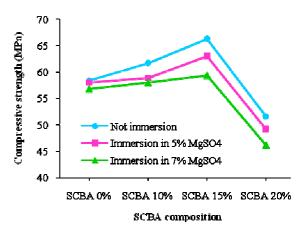
Fig. 12 The effect of SCBA composition on concrete mass with w/c = 0.300
