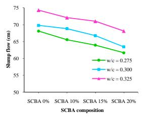
Fig. 2 The effect of SCBA on slump flow
