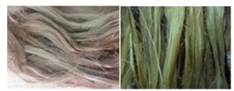
Fig. 1. Kenaf Fiber before and after treatment process
