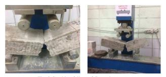
Fig. 8 Cracking failure of Control concrete
