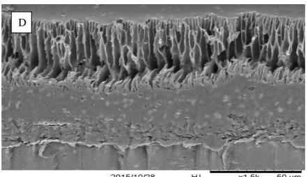
2015/10/28 H L x1.5k 50 um Fig. 4 SEM images of A) Polysulfone B) Polysulfone-PVP C) Polysulfone-TiO<sub>2</sub> D) Polysulfone-PVP-TiO<sub>2</sub> membranes under 1.5k magnification
