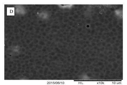
Fig. 3 SEM images of A) Polysulfone B) Polysulfone-PVP C) Polysulfone-TiO2 D) Polysulfone-PVP-TiO2 membranes under 10k magnification
