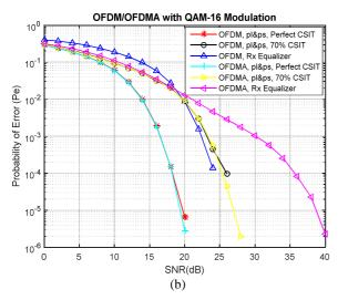
Fig. 10 The probability of error over SNRs on OFDM/OFDMA with (a) QPSK/4QAM, and (b) 16QAM Modulation.
