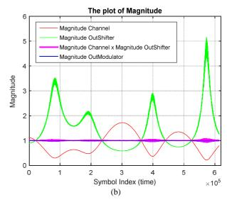
Fig. 7 (a) Magnitude channel, (b) The comparison of magnitude: magnitude channel, magnitude output shifter and magnitude output modulation
