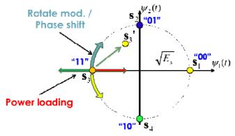
Fig. 5 Joint Power Loading and Phase SHIFTING on QPSK or 4QAM symbol (the shifting process of the symbol  $S_{11}$  to  $S_{11}^{\dagger}$ )
