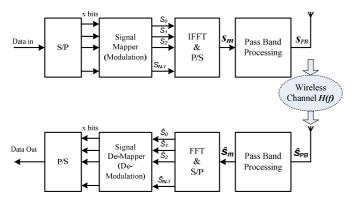
Fig. 1 FFT and inverse FFT (IFFT)-based OFDM/OFDMA systems
