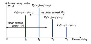
Fig. 2 The power delay profile as an excess delay function (e.g. 4 paths)
