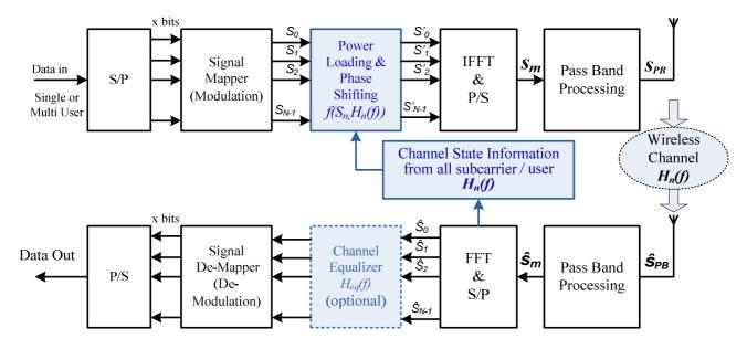
Fig. 4 Joint Power Loading and Phase Shifting OFDM/OFDMA Systems
