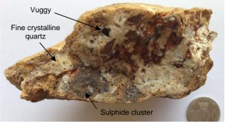
Fig. 5 Hand specimen sample of quartz vein which according to AAS assay, rich in zinc and gold (ST.07.B)
