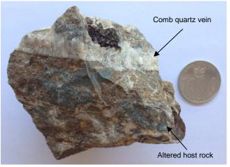
Fig. 6 Hand specimen sample showing quartz vein hosted in the altered host rock, which according to AAS assay, rich in lead and silver (ST.09.B)
