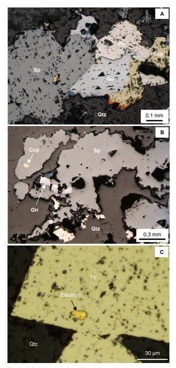
Fig. 4 Polished section photomicrographs are showing the existing ore mineral assemblages in selected mineralization samples. Fig. A, B: sphalerite (Sp), galena (Gn), chalcopyrite (Ccp), and pyrite (Py) distributed in quartz (Qtz). Fig. C: fine-grained electrum in pyrite (sample ST.12.B)
