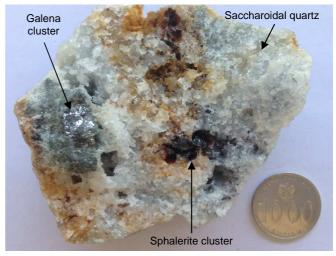
Fig. 3 Hand specimen sample of highly mineralized saccharoidal vuggy quartz from crustiform vein (sample code: ST.12.B), showing clusters of galena and sphalerite
