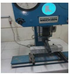
Fig. 8 Flexural test on beam
