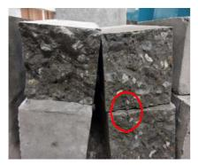
Fig. 12 Crack growth on concrete
