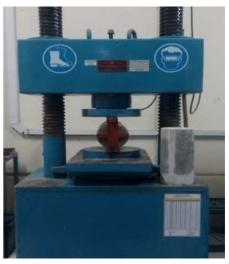
Fig. 7 Splitting tensile test on cylinder
