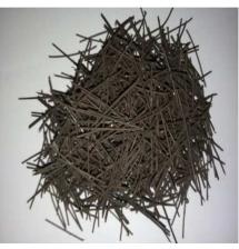
Fig. 4 The 1 inch length of steel fiber extracted from waste tyre
