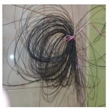
Fig. 3 Steel fiber extracted from waste tyre
