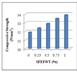
Fig. 9 Comparison of compressive strength of ordinary and SFEFWT FA concrete
