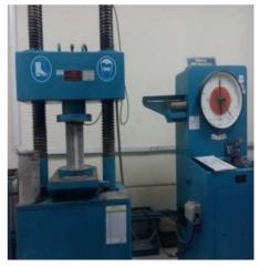
Fig. 6 Compressive test on cylinder
