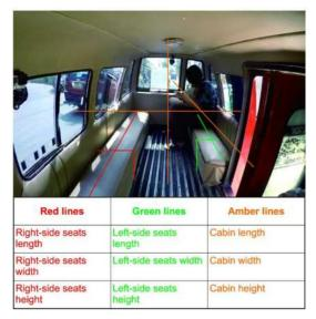
Fig. 1 Measurement framework for cabin and seating dimensions
