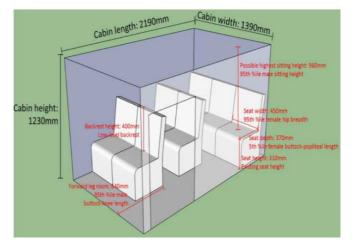
Fig. 3 Illustration of a proposed new design for angkot
