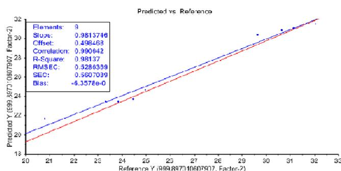
Fig. 10 Model calibration for glucose concentration prediction in *Sokan Pulau* rice according to diffuse reflectance data and chemical assay by UHPLC.
