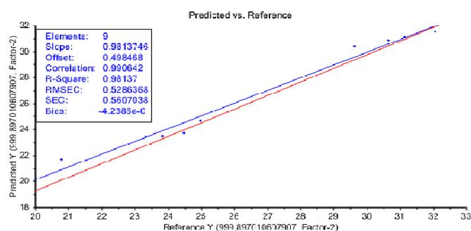
Fig. 14 Model calibration for fructose concentration prediction in *Sokan Pulau* rice according to diffuse reflectance data and chemical assay by UHPLC.
