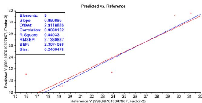
Fig. 9 Model validation for glucose concentration prediction in *Bakwan* rice according to diffuse reflectance data and chemical assay by UHPLC.
