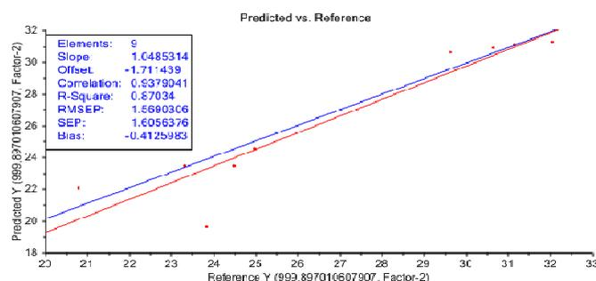
Fig. 11 Model validation for glucose concentration prediction in *Sokan Pulau* rice according to diffuse reflectance data and chemical assay by UHPLC.
