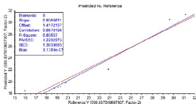
Fig. 12 Model calibration for fructose concentration prediction in *Bakwan* rice according to diffuse reflectance data and chemical assay by UHPLC.
