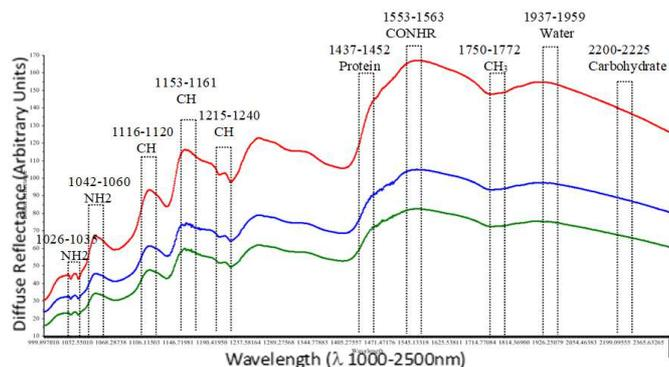
Fig. 4 Spectrum properties of *Bakwan* rice when measured using a diffused reflectance method within a 1000-2500nm wavelength. The three lines represent a quality grade of Premium (Blue), Medium (Red), and Assorted (Green).
