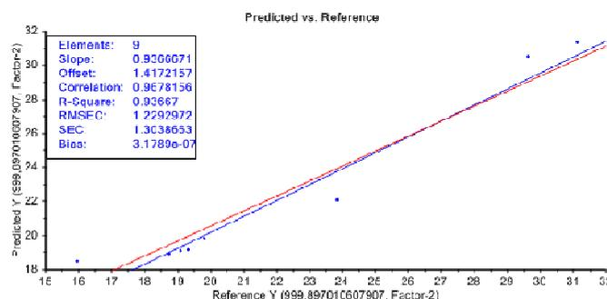
Fig. 8 Model calibration for glucose concentration prediction in *Bakwan* rice according to diffuse reflectance data and chemical assay by UHPLC.
