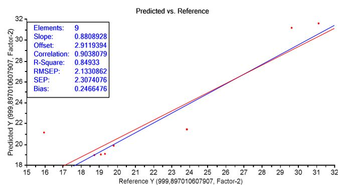
Fig. 13 Model validation for fructose concentration prediction in *Bakwan* rice according to diffuse reflectance data and chemical assay by UHPLC.
