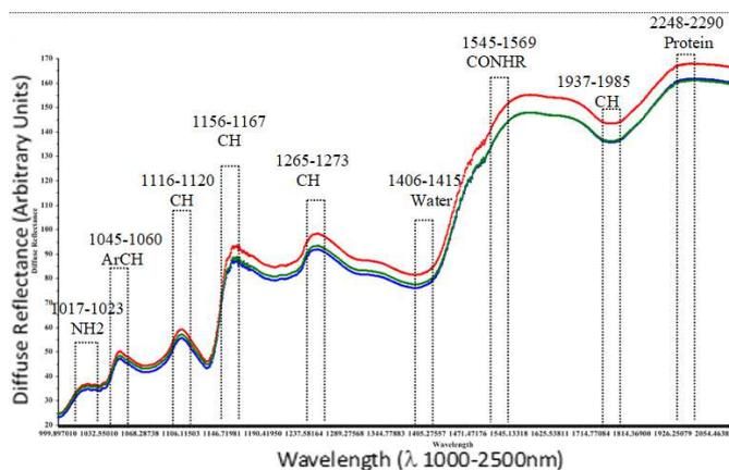
Fig. 5 Spectrum properties of *Sokan Pulau* rice when measured using a diffused reflectance method within a 1000-2500nm wavelength. The three lines represent a quality grade of Premium (Blue), Medium (Red), and Assorted (Green).
