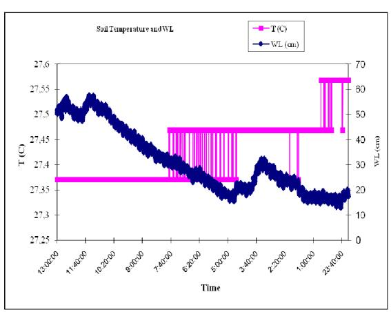
Fig. 4 Soil temperature and groundwater level measurement during the dry and wet season
