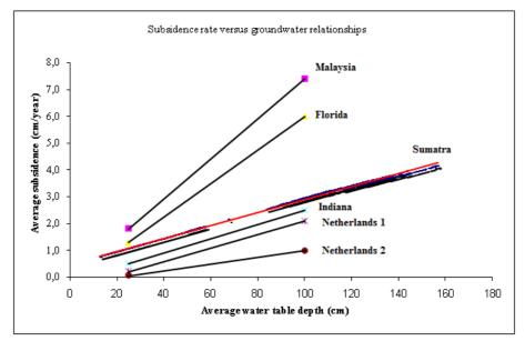
Fig.5 Land subsidence in Sumatra and around the world using Stephen equation
