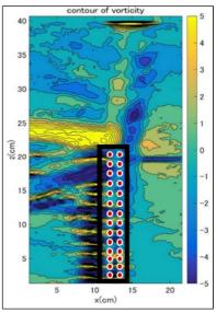
Fig. 13 Distribution map of vorticity for vegetated groyne with density 1/5, diameter 10  $\rm mm$
