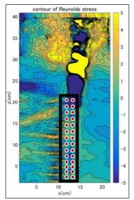
Fig. 20 Distribution map of Reynolds stress for vegetated groyne with density 1/5, diameter 10  $\rm mm$
