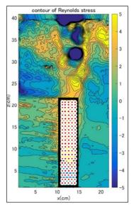
Fig. 24 Distribution map of Reynolds stress for vegetated groyne with density 1/5, diameter 5 mm
