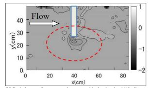
Fig. 28 Bed changes for vegetated groyne with the density 1/10, diameter 8  $\rm mm$
