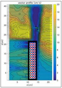
Fig. 8 Distribution map of the average flow velocity for vegetated groyne with density 1/5, diameter  $8 \mathrm{mm}$
