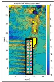
Fig. 21 Distribution map of Reynolds stress for vegetated groyne with density 1/10, diameter 8 mm
