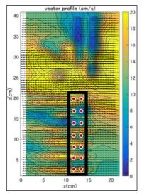
Fig. 5 Distribution map of the average flow velocity for vegetated groyne with density 1/10, diameter 10mm
