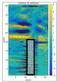
Fig. 16 Distribution map of vorticity for vegetated groyne with density 1/10, diameter 5 mm
