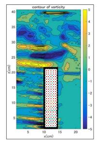
Fig. 17 Distribution map of vorticity for vegetated groyne with density 1/5, diameter 5 mm
