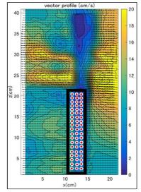
Fig. 9 Distribution map of the average flow velocity for vegetated groyne with density  $1/10,\,diameter\,5mm$
