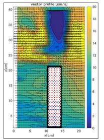
Fig. 10 Distribution map of the average flow velocity for vegetated groyne with density 1/5, diameter 5mm
