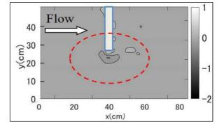
Fig. 31 Bed changes for vegetated groyne with the density 1/5, diameter 5  $\rm mm$
