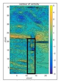
Fig. 11 Distribution map of vorticity for impermeable groyne in submerged conditions
