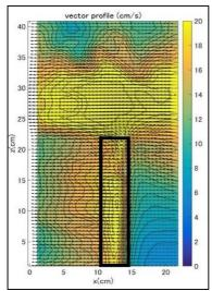
Fig. 4 Distribution map of the average flow velocity for impermeable groyne in submerged conditions
