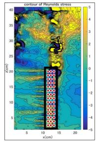
Fig. 22 Distribution map of Reynolds stress for vegetated groyne with density 1/5, diameter 8  $\rm mm$
