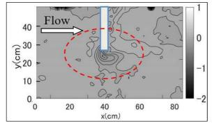
Fig. 27 Bed changes for vegetated groyne with the density 1/5, diameter 10  $\rm mm$
