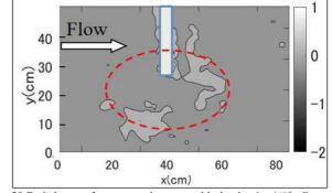
Fig. 30 Bed changes for vegetated groyne with the density 1/10, diameter 5  $\,\rm mm$
