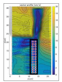
Fig. 6 Distribution map of the average flow velocity for vegetated groyne with density 1/5, diameter  $10 \mathrm{mm}$
