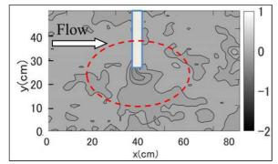
Fig. 26 Bed changes for vegetated groyne with the density 1/10, diameter 10  $\,\rm mm$
