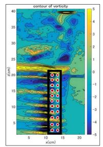
Fig. 14 Distribution map of vorticity for vegetated groyne with density 1/10, diameter 8 mm
