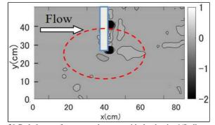
Fig. 29 Bed changes for vegetated groyne with the density 1/5, diameter 8  $\,\rm mm$
