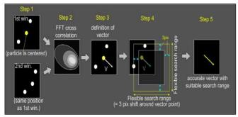
Fig. 2 The step of PTV analysis in which particle movement is obtained from two consecutive images  $% \left( {{{\rm{TV}}_{\rm{T}}}} \right)$
