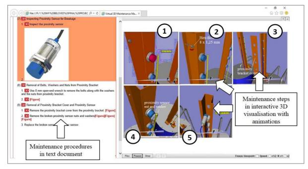
Fig. 4 Removal of the proximity sensor
