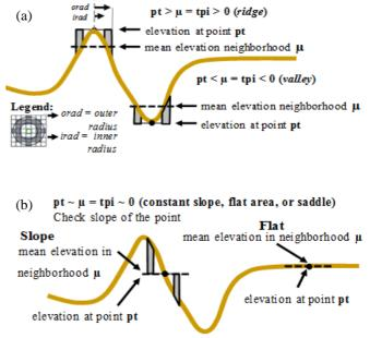
Fig. 3 Illustration for calculating topographic position index[15]
