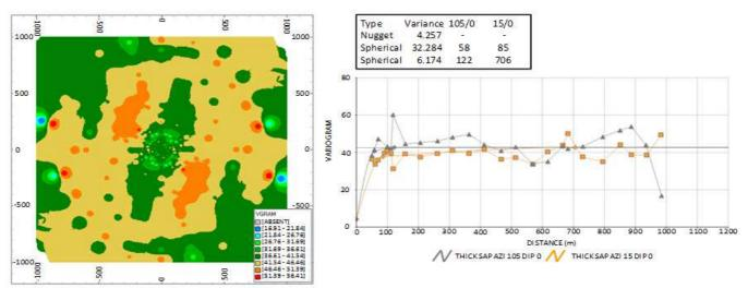
Fig. 13 Variogram map of saprolite thickness and semivariogram model along two directions
