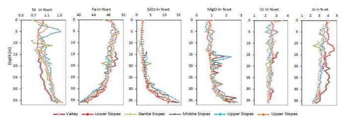
Fig. 14 Composition of Ni, Fe, SiO<sub>2</sub>, MgO, Cr and Al on limonite profile for each slope position category
