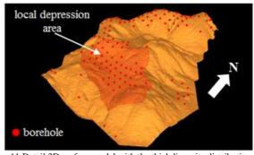
Fig. 11 Detail 3D surface model with the thick limonite distribution, showing local depression area (exaggeration z=2)
