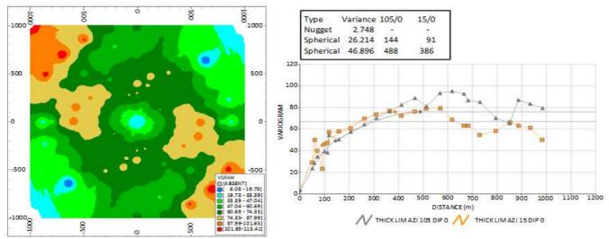
Fig. 12 Variogram map of limonite thickness and semivariogram model along two directions
