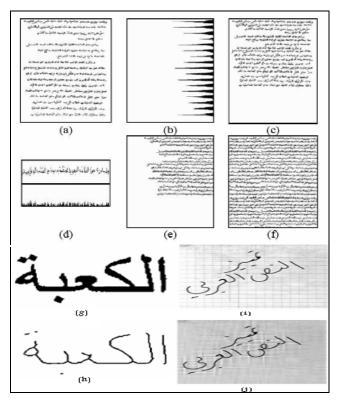
Fig. 6 Space and margin normalization (a) horizontal script (b) horizontal projection (c) line spacing normalization (d) vertical projection profile (e) word spacing normalization (f) text padding (g) The word "الكعية" before Skeletonization (h) after Skeletonization Removal of grid lines (i) original image (j) restored image [8, 9]
