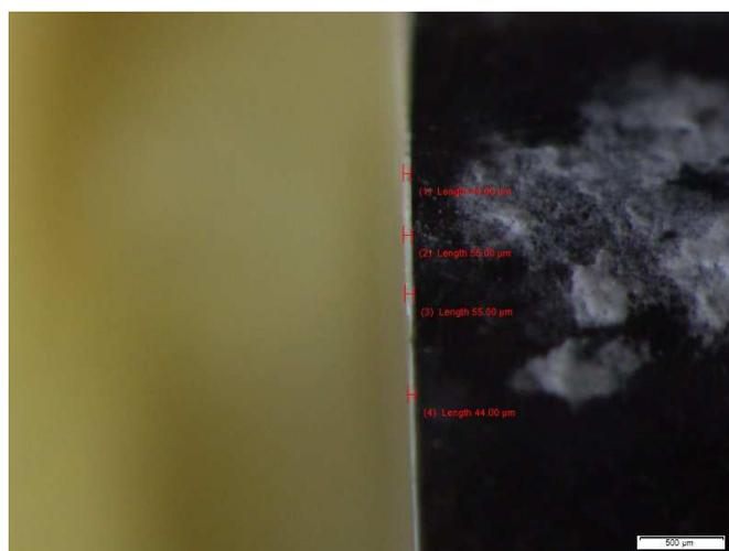
Fig. 3 Scanning electron microscope of hydroxyapatite-coated thickness at 5V for 5 minutes deposition
