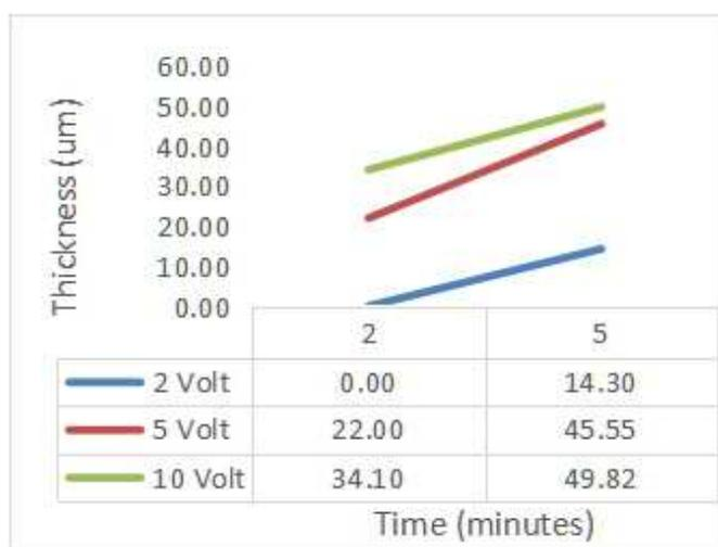
Fig. 4 Thickness curve of hydroxyapatite-coated titanium
