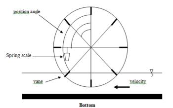
Fig 1. Spring scale use to determine moment of vane force
