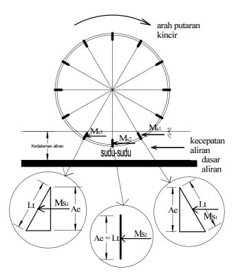
Fig 3. Area of vane toward water flow at different vane position angle
