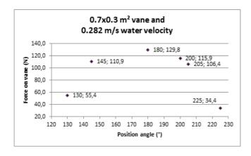
Fig 2. Force on single vane for different vane position angle
