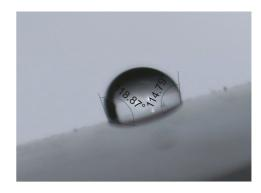
Fig. 8 The contact angle being formed by a water droplet on the surface of a silicone-rubber post-insulator
