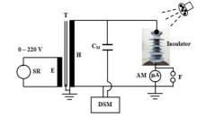
Fig. 3 The experimental set-up for leakage current observation
