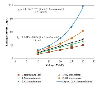
Fig. 4 The relationship between the applied voltage and the leakage current of insulator in dry and wet conditions
