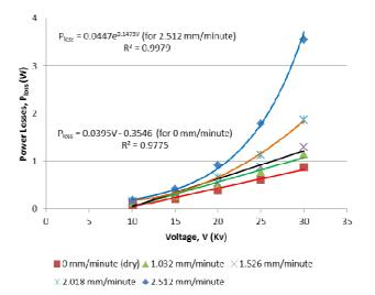
Fig. 6 The relationship between the power losses and the applied voltage for each wetting intensity
