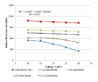
Fig. 5 The relationship between the surface resistance and the applied voltage for each wetting intensity
