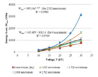
Fig. 7 The relationship between the annual energy losses and the applied voltage for each wetting intensity
