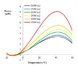
Fig. 9 Power versus temperature at various solar irradiances at  $90^\circ$  solar angle of the non-laminated solar module
