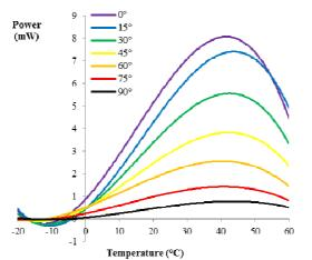
Fig. 11 Power versus temperature at a various solar angle at 350W/m<sup>2</sup> of the non-laminated solar module
