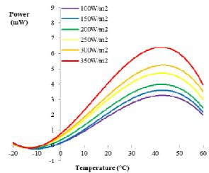
Fig. 10 Power versus temperature at various solar irradiances at  $90^\circ$  solar angle of the laminated solar module
