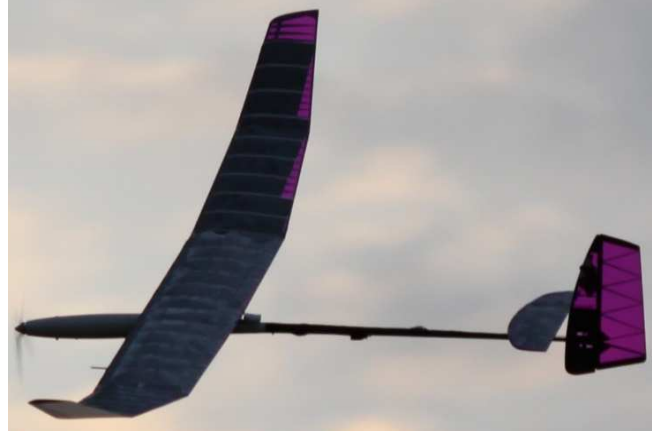
Fig. 2 Solar-powered UAV developed Aircraft Design Group, Cranfield University
