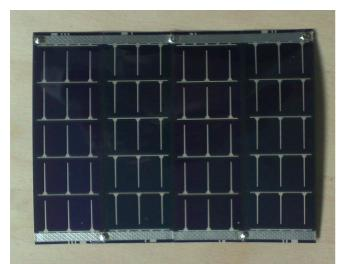
Fig. 1 The fabricated 12 V solar module
