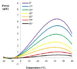
Fig. 12 Power versus temperature at a various solar angle at 350W/m<sup>2</sup> of the non-laminated solar module
