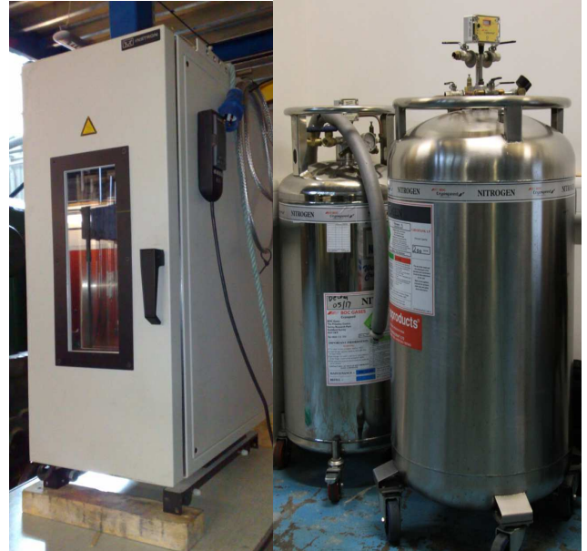
Fig. 5 Environmental testing chamber with a liquid nitrogen tank
