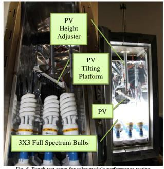
Fig. 6 Bench test setup for solar module performance testing
