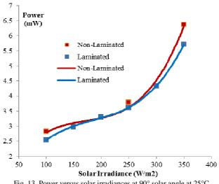
Fig. 13 Power versus solar irradiances at 90° solar angle at 25°C
