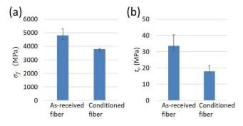
Fig. 5 Fiber strength (a) and interfacial strength (b) for the as-received and conditioned fibers [10]
