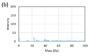
Fig. 4 TOF-SIMS spectra for the as-received fibers (a) and conditioned fibers (b). The decreased intensity of peaks in the range from 20 to 60 Da indicates that the hydrocarbon at the interface was eliminated
