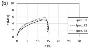
Fig. 6 Stress-strain curves of the as-received fiber-epoxy composite (a) and the conditioned fiber-epoxy composite (b) tested under transverse loading
