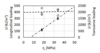
Fig. 9 Toughness of the composite versus interfacial strength
