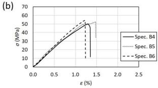
Fig. 7 Stress-strain curves of the as-received fiber-epoxy composite (a) and the conditioned fiber-epoxy composite (b) tested under longitudinal loading
