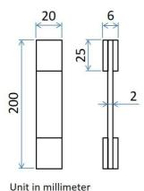
Fig. 2 Schematic showing the specimen dimensions
