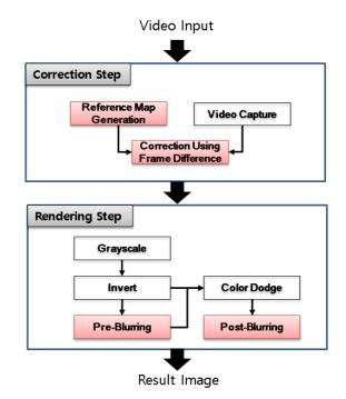
Fig. 4 The overview of suggested video based sketch rendering system.
