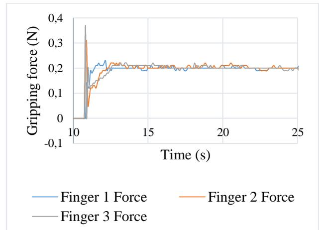
Fig. 4 Steady state response of gripping of 100g mass
