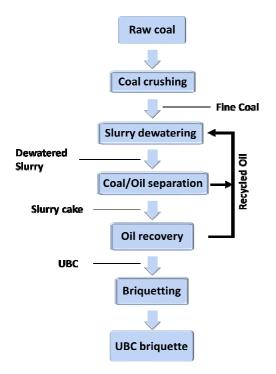
Fig. 4 Block diagram of Upgrading Brown Coal (UBC) process
