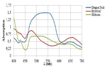
Fig. 11 Absorption of single dye with UV-Vis Spectrophotometer
