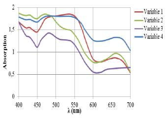
Fig. 12 Absorption of multiple dyes with UV-Vis Spectrophotometer
