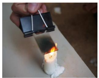
Fig. 6 Carbon electrode from wax candle sintering
