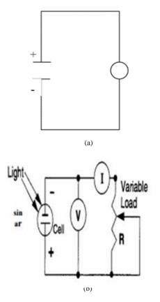
Fig. 12 (a) Open circuit, (b) Closed circuit
