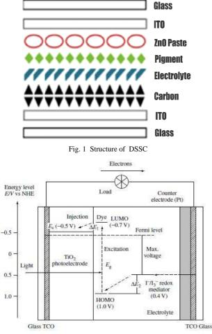
Fig. 2 Schematic energy diagram and operating principle of DSSC
