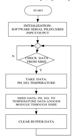
Fig. 2 Flowchart program Arduino Uno
