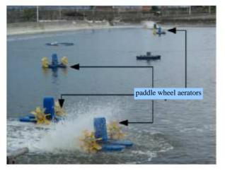
Fig. 9 Aeration system consisting of many paddle wheel aerators operated automatically based on the DO value of the water
