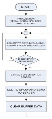
Fig. 5 Flowchart program data logger module
