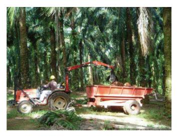
Fig. 5 Small-size farm machinery for oil palm FFB evacuation [17].
