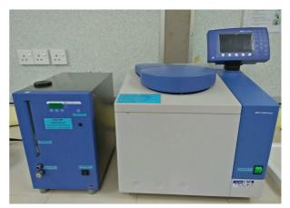
Fig. 2 Bomb Calorimeter C 2000 Basic
