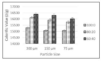
Fig. 6 Effect of particle size with different mixing ratio on calorific value
