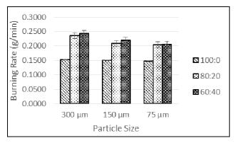
Fig. 5 Effect of particle size with different mixing ratio on burning rate
