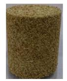
Fig. 1 Biomass composite briquette produced
