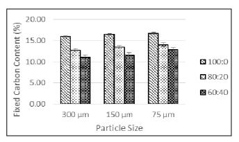
Fig. 9 Effect of particle size with different mixing ratio on the fixed carbon content
