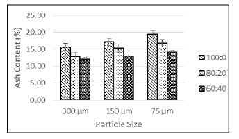
Fig. 7 Effect of particle size with different mixing ratio on ash content
