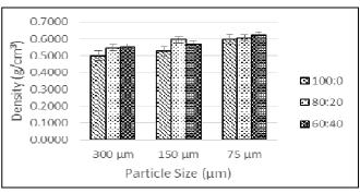
Fig. 3 Effect of particle size with different mixing ratio on density
