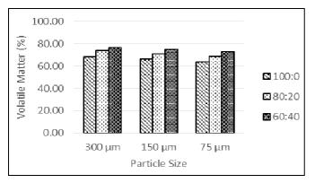
Fig. 8 Effect of particle size with different mixing ratio on volatile matter
