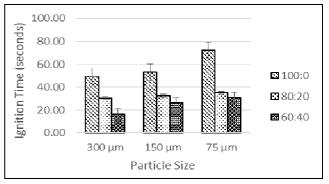
Fig. 4 Effect of particle size with the different mixing ratio of ignition time
