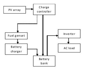
Fig. 1 Block diagram of HSAPV system
