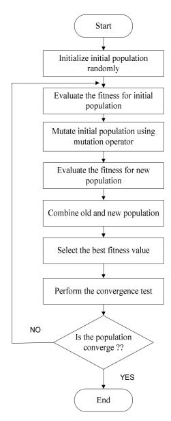
Fig. 2 Flowchart of evolutionary programming (EP).
