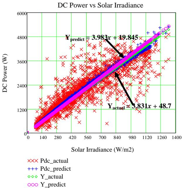
Fig. 4 DC Power versus solar irradiance (Polycrystalline)
