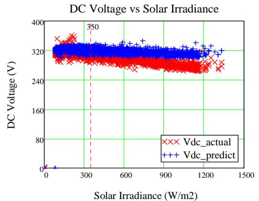
Fig. 7 DC Voltage versus solar irradiance (Polycrystalline)
