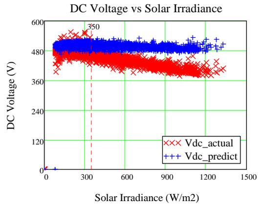
Fig. 5 DC Voltage versus solar irradiance (Monocrystalline)
