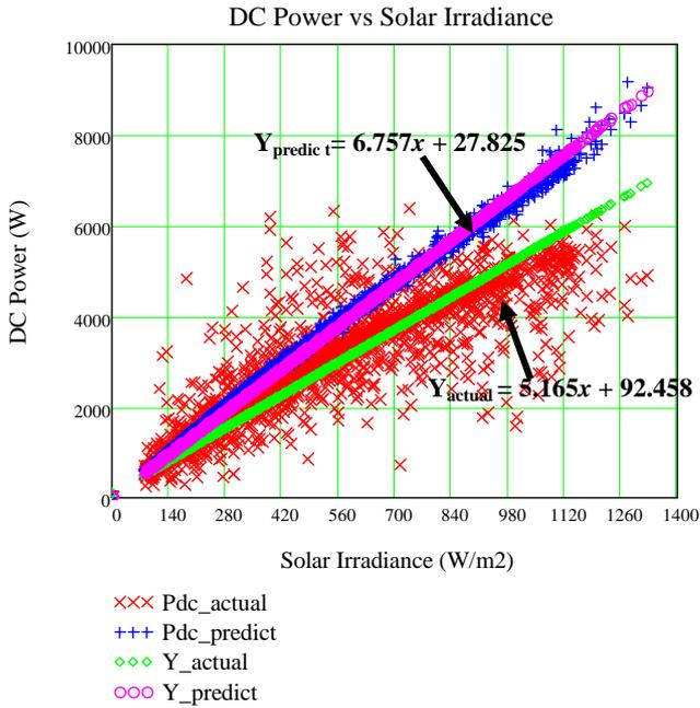
Fig. 3 DC power versus solar irradiance (Monocrystalline)
