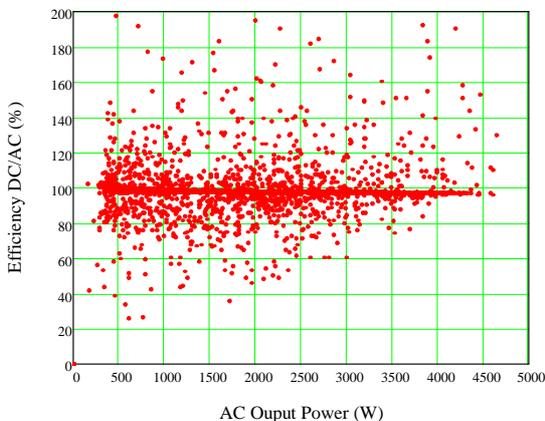
Fig. 14 The relationship between the inverter efficiency and AC output power (Polycrystalline)
