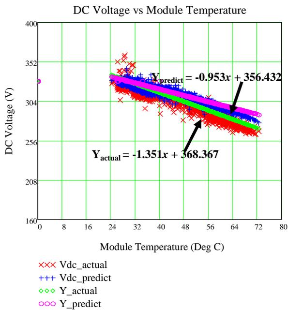
Fig. 8 DC Voltage versus module temperature (Polycrystalline)
