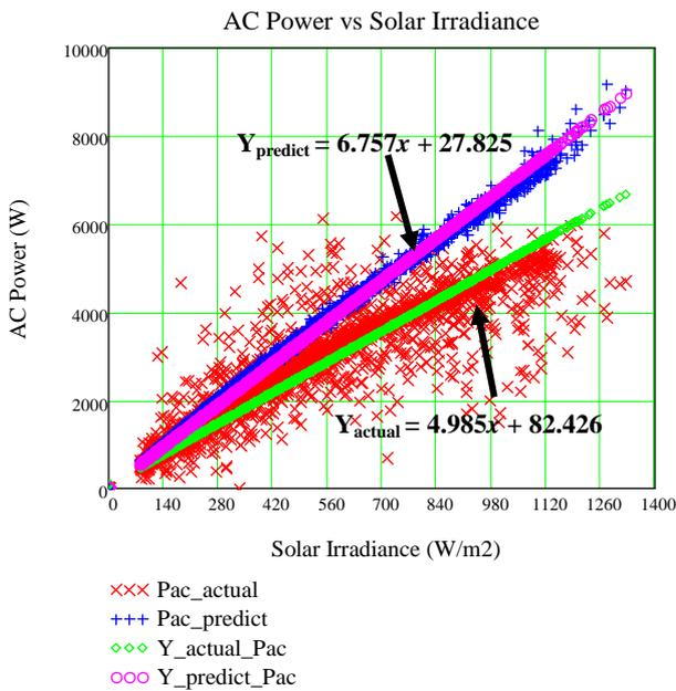
Fig. 12 AC Power versus solar irradiance (Monocrystalline)
