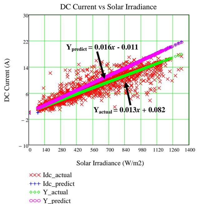
Fig. 10 DC Current versus solar irradiance (Polycrystalline)
