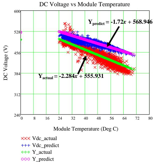
Fig. 6 DC Voltage versus module temperature (Monocrystalline)
