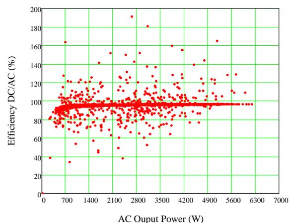
Fig. 11 The relationship between the inverter efficiency and AC output power (Monocrystalline)
