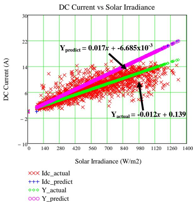
Fig. 9 DC Current versus solar irradiance (Monocrystalline)
