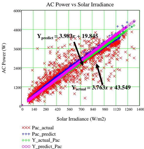
Fig. 13 AC Power versus solar irradiance (Polycrystalline)
