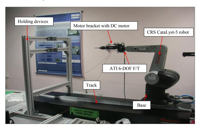
Fig. 5 Real layout drilling operation
