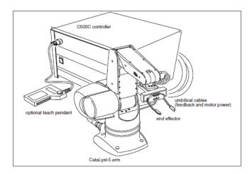
Fig. 1 Basics component of CRS
