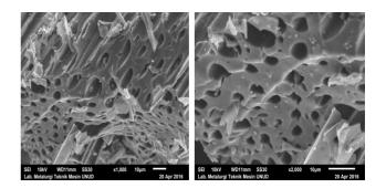
Fig. 1 SEM bamboo biochar
