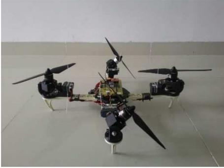
Fig. 6 Prototype of quad tiltrotor
