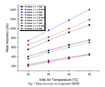
TABLE III AMOUNT OF HEAT RECOVERY ON EVAPORATOR HPHE
