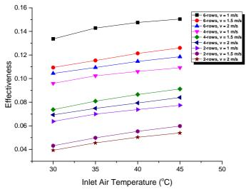
Fig. 6 The effectiveness of heat pipe heat exchanger
