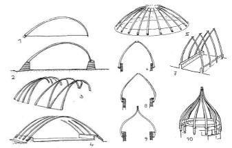
Fig. 2 Bamboo arch structure [16]
