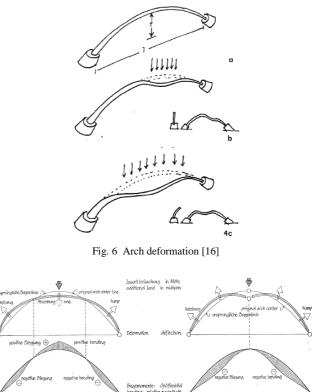
Fig. 7 Arch deflection and bending moment diagram [22]
