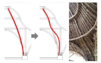
Fig. 15 Buckling at main curved column
