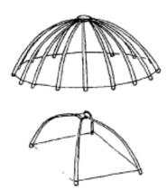
Fig. 3 Centralized configuration of bamboo curved elements [16]
