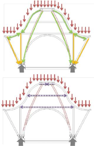
Fig. 13 Gravitational load distribution. meridional force (top) and hoop force (bottom).
