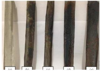
Fig. 2 SS 316 (a) without pretreatment, (b) 1 minute, (c) 5 minutes, (d) 10 minutes, and (e) 20 minutes of pretreatment
