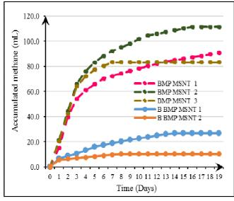
Fig. 2 Cumulative methane production from digesting DMSS; organic content of  $0.52\,$
