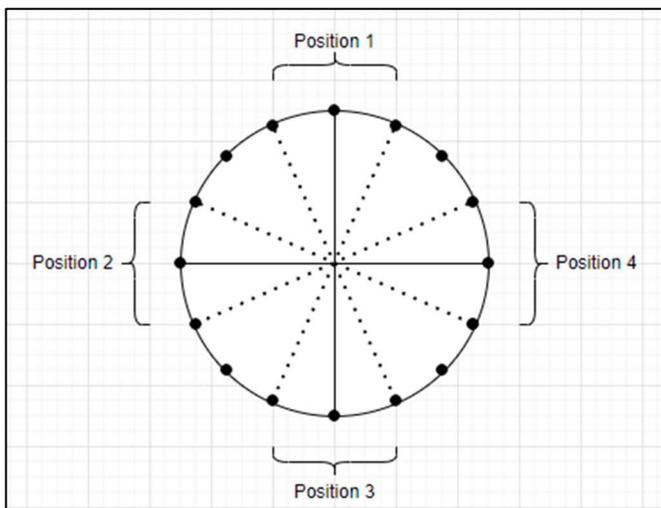
Fig. 5 Top view of capacitive sensors structure
