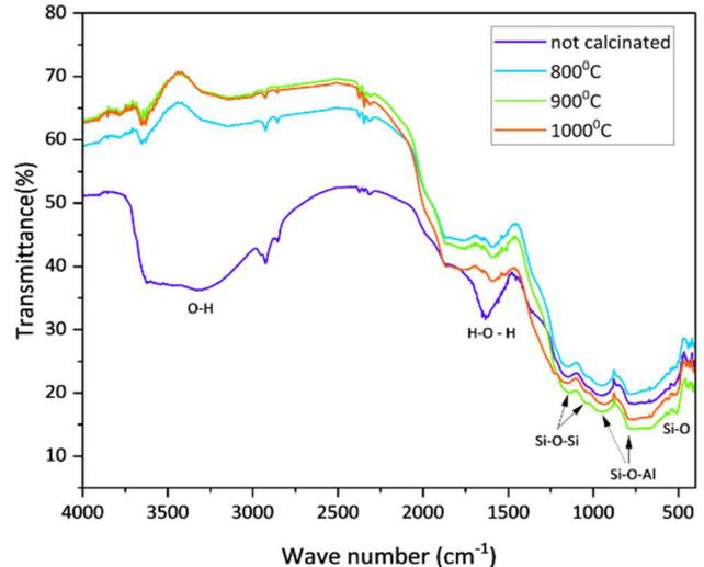
Fig. 6 FTIR spectra of volcanic ash
