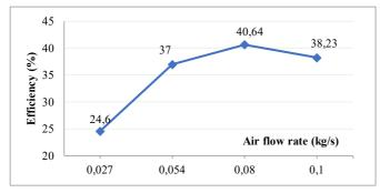
Fig. 10 The efficiency of flat plate solar collector with air flow rate difference
