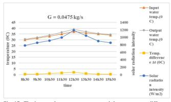
Fig. 17 The input and output temperature and the temperature difference following the solar radiation intensity for the case of water 0.00475 kg/s
