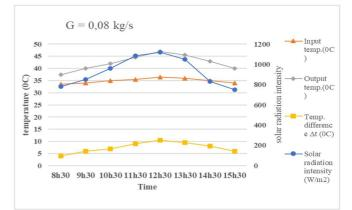
Fig. 9 The input and output temperature and the temperature difference following the solar radiation intensity for the case of 0.08 kg/s.
