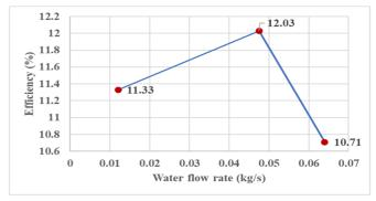
Fig. 18 The efficiency of the solar collector with glass tubes placed at the focal point of the parabolic trough with water flow rate difference.
