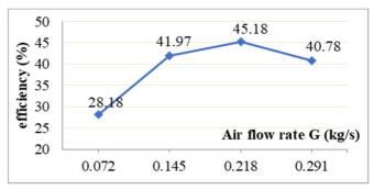
Fig. 20 The efficiency of the solar collector using the heat collector tube placed at the focal point of the parabolic cylinder (without expanding the receiver surface area).
