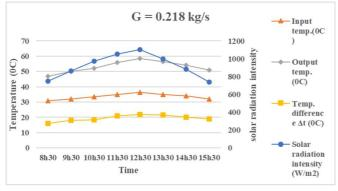
Fig. 21 The input and output temperature and the temperature difference following the solar radiation intensity for the case of 0.218 kg/s
