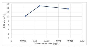
Fig. 14 The efficiency of the solar collector using copper tubes placed at the focal point of the parabolic trough with different water flow rate.
