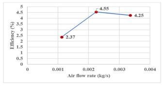
Fig. 16 The efficiency of the solar collector with glass tubes placed at the focal point of the parabolic trough tested with air at three different air flow rates: 0.00112 kg/s, 0.00224 kg/s, and 0.00336 kg/s.
