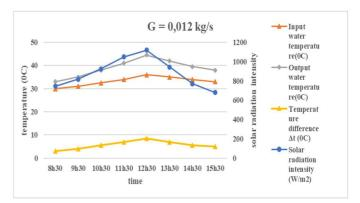
Fig. 13 The input and output water temperature and the temperature difference following the solar radiation intensity for the case of 0.012 kg/s.
