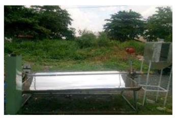
Fig. 6 The glass tube collector placed on the focus of a parabola surface.
