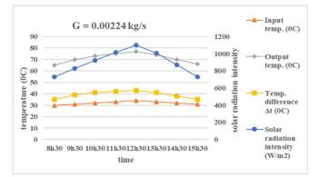
Fig. 15 The input and output temperature, and the temperature difference following the solar radiation intensity for the case of 0.00224 kg/s
