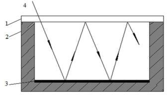
Fig. 2 Structure of a flat plate solar collector (1. Glass panels; 2. Insulation shell; 3. Absorber plate; 4. Solar radiation)
