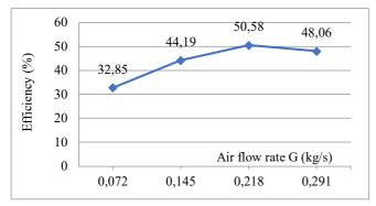
Fig. 22 The efficiency of solar collector using the heat collector tube placed at the focal point of the parabolic cylinder (with expanding the receiver surface area).
