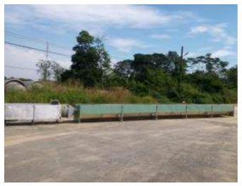
Fig. 7 The pipe collector placed on the focus of the parabolic cylinder with no extent the collector (the parabola is insulated)
