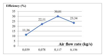
Fig. 12 The efficiency of solar tube collectors made of transparent polyethylene thin film with air flow rate difference.
