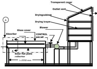
Fig. 1 Schematic of a solar dryer [32]
