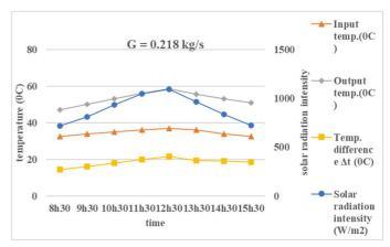
Fig. 19 The input and output temperature and the temperature difference following the solar radiation intensity for the case of 0.218 kg/s
