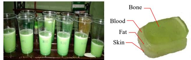
Fig. 14 Manufacture and modeling of gelatin as an artificial finger tissue
