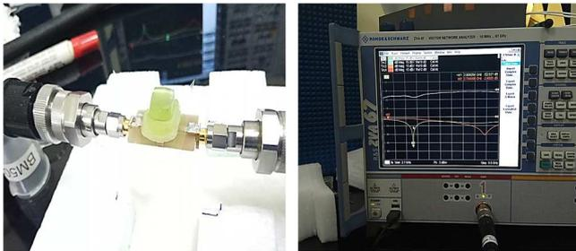
Fig. 17 Installation of measurements of CPW sensors loaded with SRR-IDCC using VNA (with test material)
