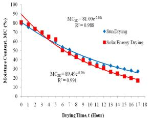
Fig. 3. Fish moisture content plotted against drying time for both the solar drying and the sun drying
