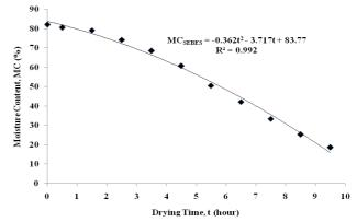
Fig. 9. Fish moisture content plotted against drying time for the biomass energy drying for the simultaneous solar energy and biomass energy drying
