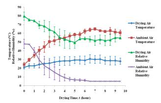
Fig. 8. Drying air temperature, ambient air temperature, drying air relative humidity, ambient air relative humidity plotted against drying time for the simultaneous solar energy and biomass energy drying
