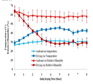
Fig. 2. Daily temperature and relative humidity plotted against daily drying time for both the solar energy drying and the sun drying
