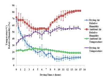
Fig. 6. Drying air temperature, ambient air temperature, drying air relative humidity, ambient air relative humidity plotted against drying time for the solar energy drying continued by the biomass energy drying
