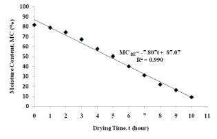
Fig. 5. Fish moisture content plotted against drying time for the biomass energy drying
