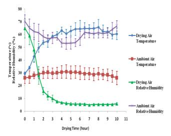
Fig. 4. Drying air temperature, ambient air temperature, drying air relative humidity, ambient air relative humidity plotted against drying time for the biomass energy drying
