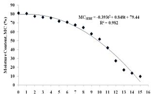
Fig. 7. Fish moisture content plotted against drying time for the biomass energy drying for the solar energy drying continued by the biomass energy drying
