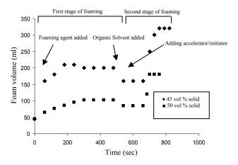
Fig. 1. Foam volume generated in two stages, using ethanol as organic solvent.
