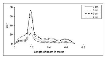
Fig.14 CDF for beam having different crack depths at 0.25L
