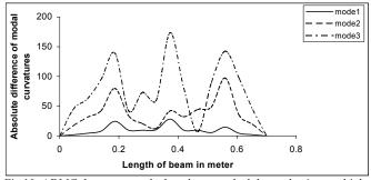
Fig.10 ADMC between cracked and un-cracked beam having multiple cracks of 5 cm depth at 0.25L, 0.5L and 0.75L
