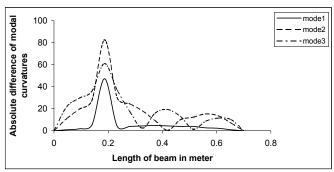
Fig.6 ADMC between cracked and un-cracked beam having crack of 5  $\it cm$  depth at 0.25L
