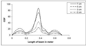
Fig.13 CDF for beam having different crack depths at 0.5L
