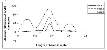
Fig.2 ADMC between cracked and un-cracked beam having crack of 5  $\it cm$  depth at 0.5L
