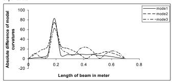
Fig.5 ADMC between cracked and un-cracked beam having crack of 7 cm depth at 0.25L
