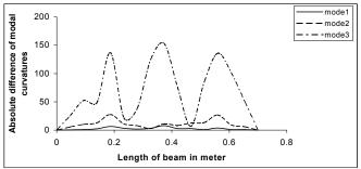
Fig.12 ADMC between cracked and un-cracked beam having multiple cracks of 2 cm depth at 0.25L, 0.5L and 0.75L
