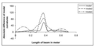
Fig.1 ADMC between cracked and un-cracked beam having crack of 7 cm denth at 0.5L.
