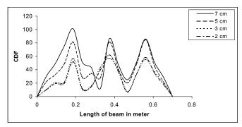
Fig.15 CDF for beam having different crack depths at 0.25L, 0.5L and  $0.75 L\,$
