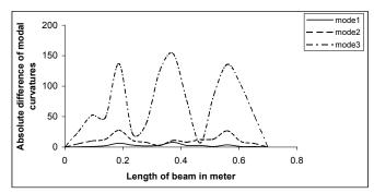
Fig.11 ADMC between cracked and un-cracked beam having multiple cracks of 3 cm depth at 0.25L, 0.5L and 0.75L
