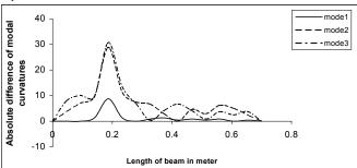
Fig.8 ADMC between cracked and un-cracked beam having crack of 2  $\it cm$  depth at 0.25L
