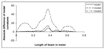
Fig.4 ADMC between cracked and un-cracked beam having crack of 2  $\it cm$  depth at 0.5L
