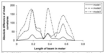
Fig.9 ADMC between cracked and un-cracked beam having multiple cracks of  $7\ cm$  depth at 0.25L, 0.5L and 0.75L
