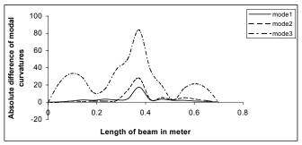
Fig.3 ADMC between cracked and un-cracked beam having crack of 3  $\it cm$  depth at 0.5 L
