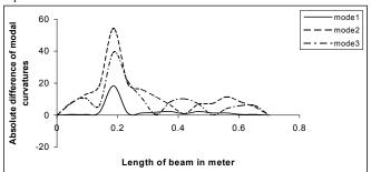
Fig.7 ADMC between cracked and un-cracked beam having crack of 3  $\it cm$  depth at 0.25L
