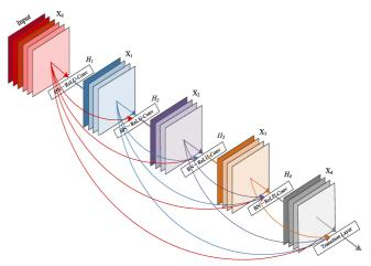
Fig. 4 The architecture of the DenseNet201 model [21]
