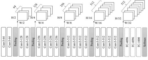
Fig. 3 The architecture of the VGG19 model [19]
